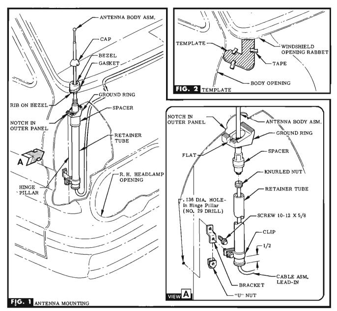
STEP 1 ALIGN TEMPLATE ON RIGHT HAND BODY FRONT OUTER PANEL, TAPE IN PLACE, CENTER PUNCH & DRILL AS INDICATED ON TEMPLATE. REMOVE ANY RESULTANT BURRS. SEE FIG. 2.
