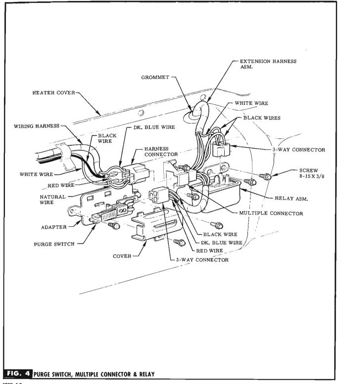
STEP 19 SUB ASSEMBLE PURGE SWITCH & COVER TO ADAPTER WITH SCREWS (IN BAG A). SEE FIG. 4.
