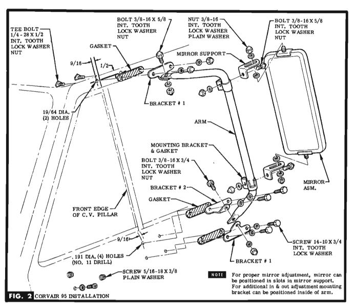
STEP 10 ON L. H. SIDE ONLY, REMOVE & DISCARD EXIST-ING MIRROR & ATTACHING PARTS. PLUG HOLES WITH PARTS PROVIDED. SEE FIG. 2.
