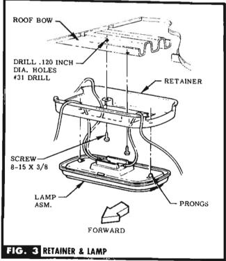
STEP 7 POSITION RETAINER ON CENTER OF REAR ROOF BOW & USE IT AS A TEMPLATE TO DRILL HOLES. SEE FIG. 3. CAUTION Do not drill thru roof panel.
