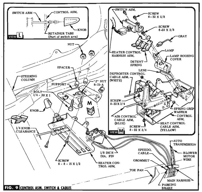
STEP 46 INSERT LENS INTO SLOT IN CONTROL & POSITION COVER, DETENT SPRING, SWITCH & SECURE WITH SCREWS (IN BAG A). SEE VIEW M.
