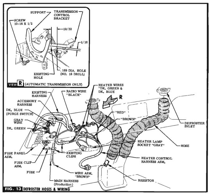
STEP 67 (IF AUTOMATIC TRANSMISSION EXISTS) INSTALL HOSE SUPPORT ON TRANSMISSION CONTROL BRACKET WITH SCREW PROVIDED (IN BAG A). SEE VIEW R.
