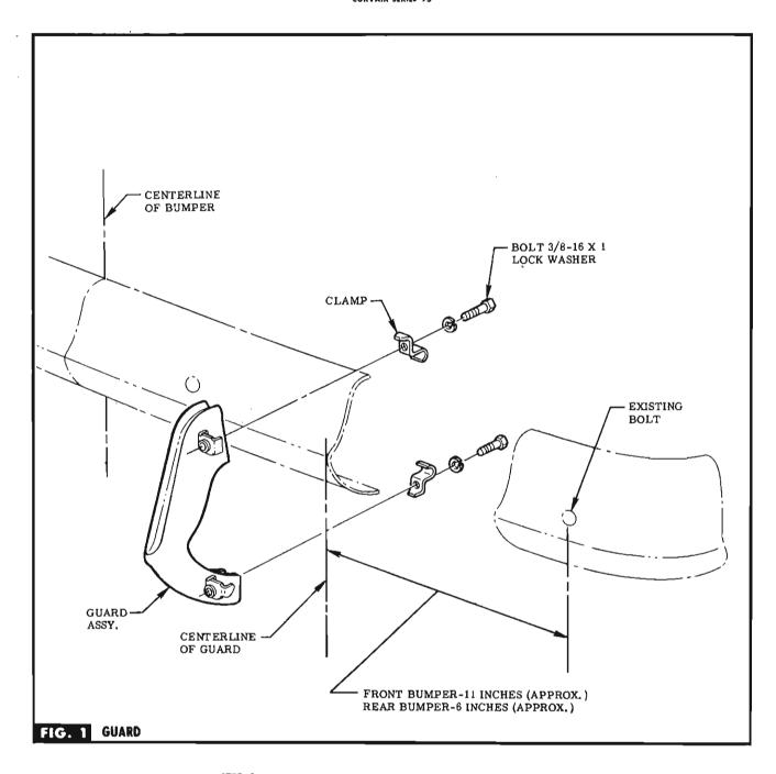
**STEP 1** INSTALL GUARD ON FRONT OR REAR BUMPER AT LOCATION SHOWN WITH ATTACHING PARTS PROVIDED, UPPER & LOWER BOLTS SHOULD BE TIGHTENED PROGRESSIVELY TO INSURE PROPER FIT. SEE FIG. 1,
