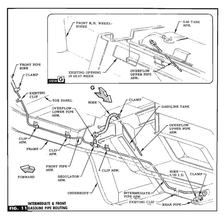
STEP 47 ROUTE INTERMEDIATE PIPE FORWARD ALONG EX-ISTING PIPE, ATTACHING TO FRAME WITH EXISTING & PROVIDED CLIPS (IN BAG C). SEE FIG. 11.
