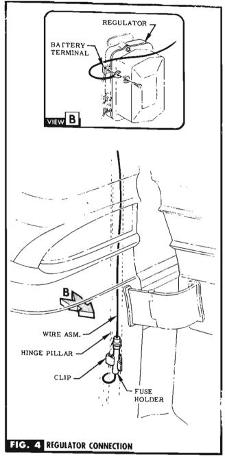
assist routing thru holes & around corners.
