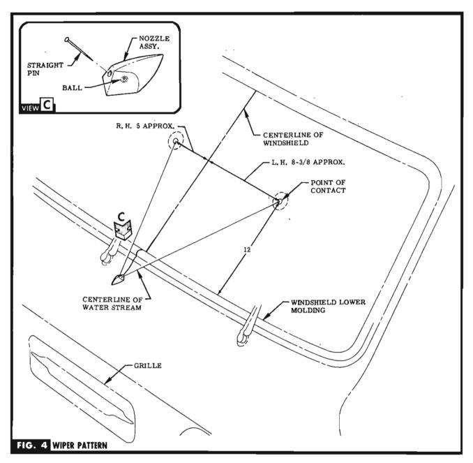
**STEP 11** TEST SYSTEM TO INSURE CORRECT INSTALLATION & DETERMINE LOCATION OF POINT OF CONTACT FOR WATER STREAM. SEE FIG. 4.
