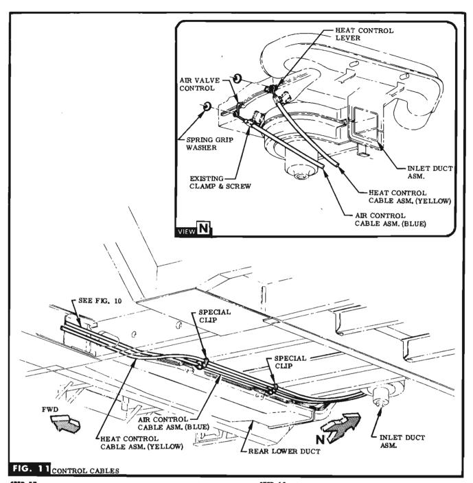
STEP 57 INSTALL CLIPS (IN BAG B) TO INTERMEDIATE & REAR CROSSMEMBERS ALONG SIDE DUCT SECURING SCREWS, SEE FIG. 11.
