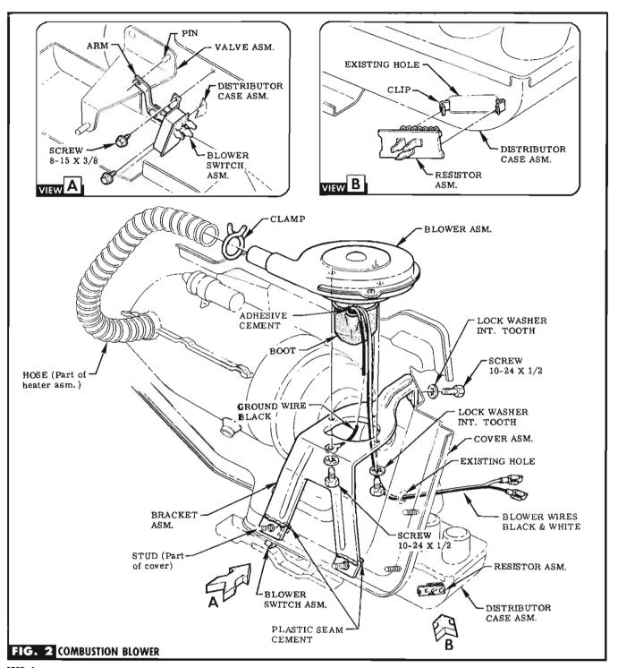
**STEP 6** PLACE BLOWER SWITCH ARM ON VALVE PIN & ATTACH TO DISTRIBUTOR CASE WITH ATTACHING SCREWS PROVIDED (IN BAG A). SEE VIEW A.
