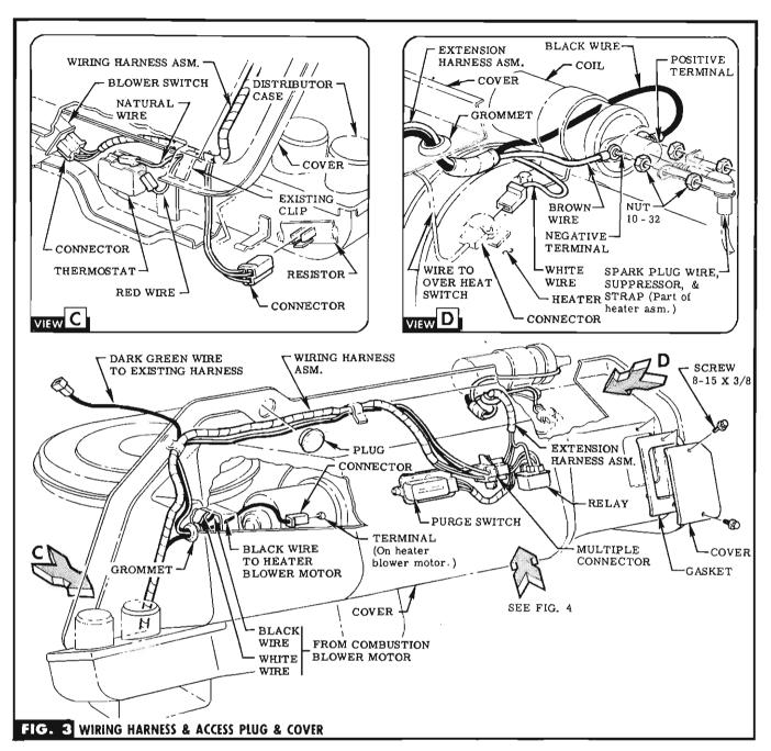
STEP 12 PLUG HARNESS CONNECTORS ONTO BLOWER SWITCH & RESISTOR. SEE VIEW C.
