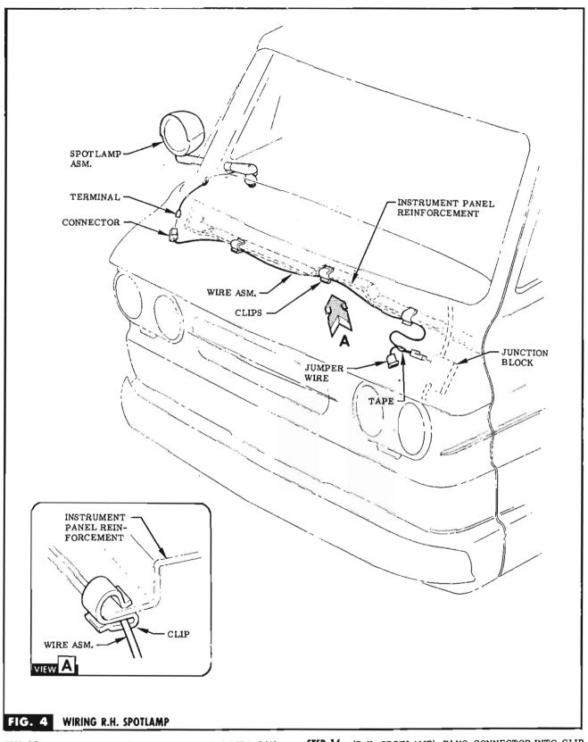
STEP 15 (R.H. SPOTLAMP) PLUG TERMINAL INTO CONNECTOR ON WIRE ASM. INSTALL CLIPS ON INSTRUMENT PANEL REINFORCEMENT AT CONVENIENT LOCATIONS. ROUTE WIRE ASM, THRU CLIPS. SEE FIG. 4 & VIEW A.
