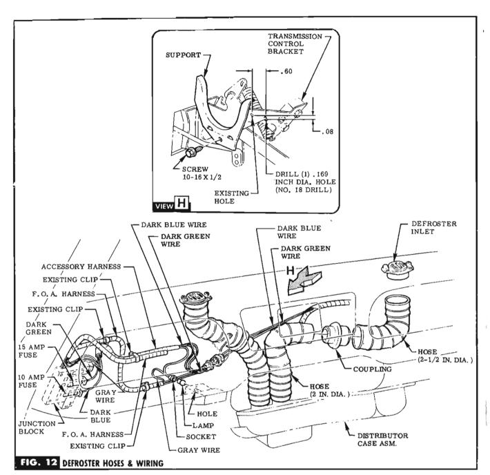
**STEP 58** IF AUTOMATIC TRANSMISSION EXISTS, DRILL HOLE & INSTALL HOSE SUPPORT ON TRANSMISSION CONTROL BRACKET WITH SCREW (IN BAG A). SEE VIEW. H.
