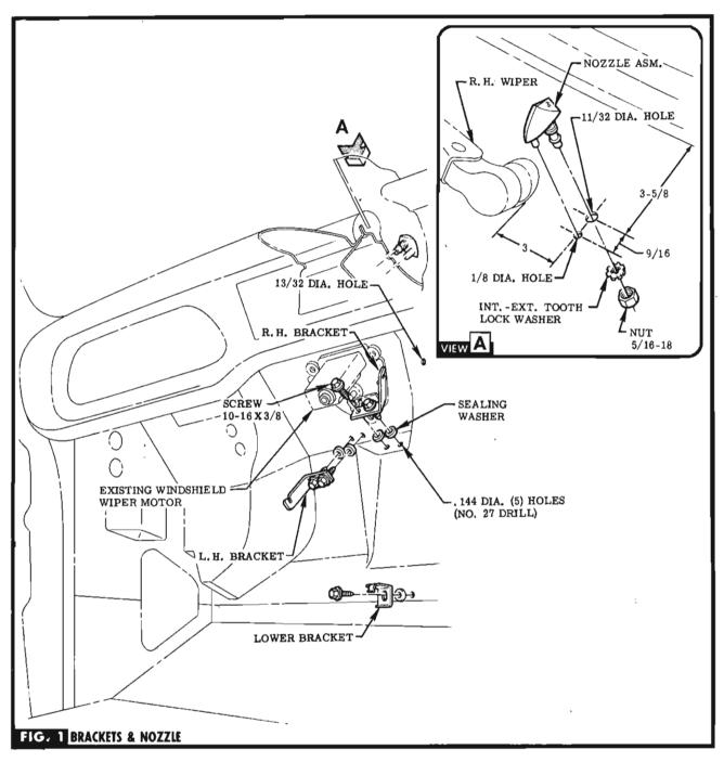
STEP 1 LOCATE EXISTING DIMPLES IN DASH PANEL & DRILL HOLES FOR UPPER R. H. & L. H. & LOWER BRACKETS & GROMMET. SEE FIG. 1. NOIL II heater exists, use lower hole of heater control cables clip for attaching lower bracket.
