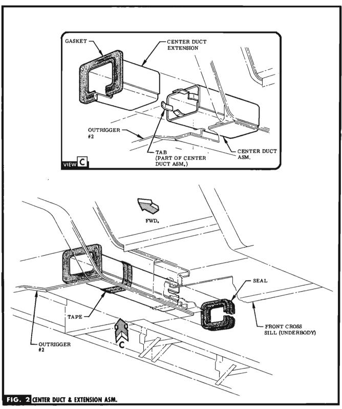
STEP 9 INSTALL GASKET ONTO CENTER DUCT EXTENSION. SEE VIEW  $\mathbf{C}_{\bullet}$
