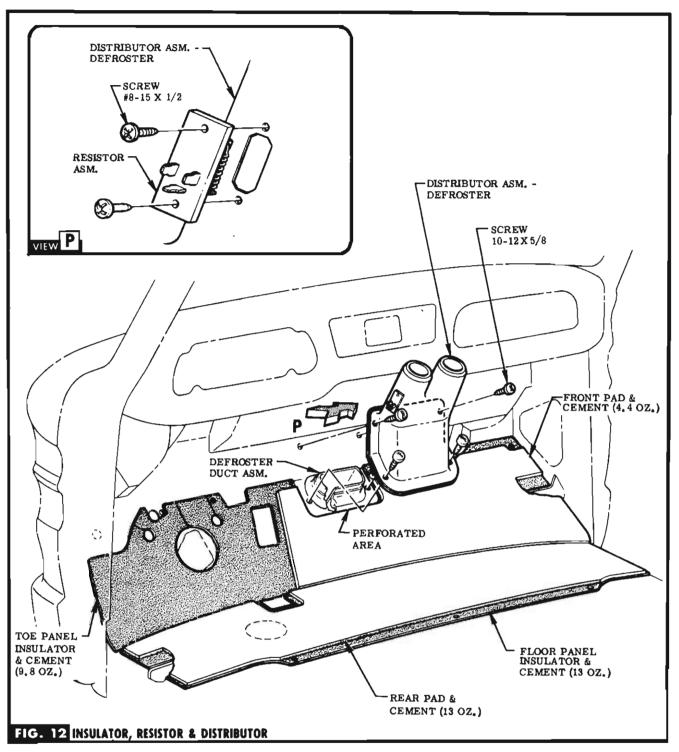
STEP 63 REMOVE EXISTING FLOOR MAT & CEMENT PROVIDED PADS TO UNDERSIDE OF FLOOR MAT. CUT OUT PERFORATED AREA. SEE FIG. 1.
